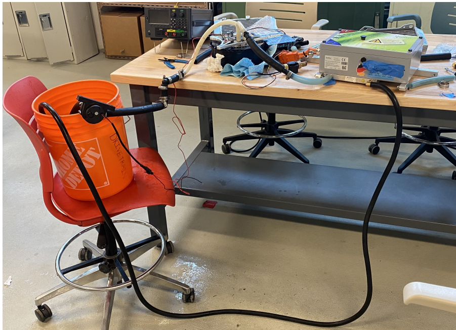
Figure 30: The Liquid Flow Rate Test Setup
